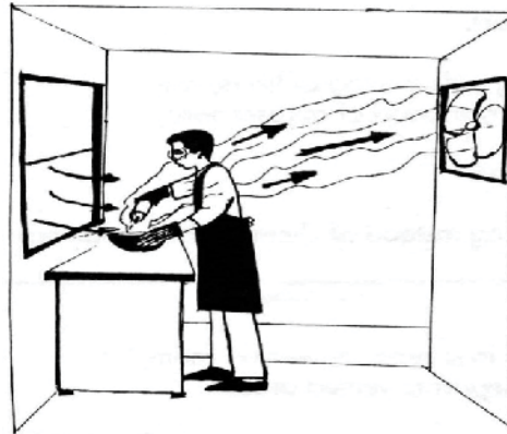
Bad ventilation: Outside air from the open window blows the chemicals into the worker's face before being vented out of the salon.
