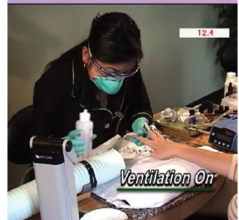
Ventilation on: With a ventilation system running, chemical levels dropped significantly during the same process (below 12.4 parts per million).
